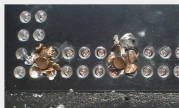
Even 40 caliber bullets fired from point blank range could not penetrate the armored Radarsign Bashplate™ or do massive internal damage to the sign.
